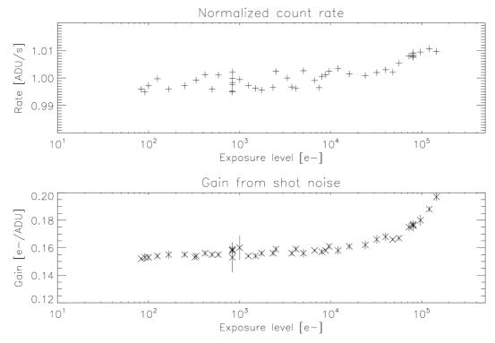
Illustration 1: Output A. Data merged from two sequences at different illumination levels.
