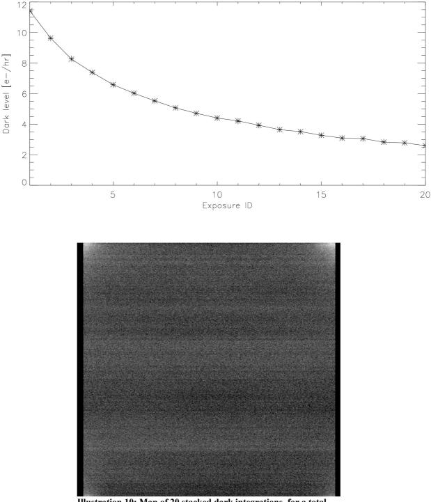
Illustration 10: Map of 20 stacked dark integrations, for a total integration time of 10 hours. The image area is clearly brighter than the overscan region, and brightest near the corners. Horisontal bands appear due to bias level fluctuations.
