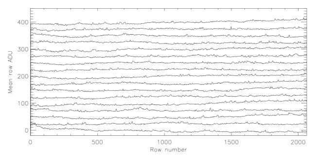
Illustration 11: Vertical profiles of 17 full-frame biases. A separation of 25 ADU between profiles has been added.
