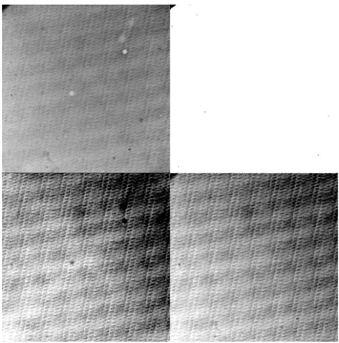
Illustration 6: 334nm flat fields. Lower left: May 2015. Lower right: March 2016. Both displayed with +/- 10% grey-scale cuts. Upper left: Ratio of the two flats, displayed with +/- 5% grey-scale cuts.
