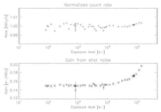
Illustration 3: Output C. Data merged from two sequences at different illumination levels.
