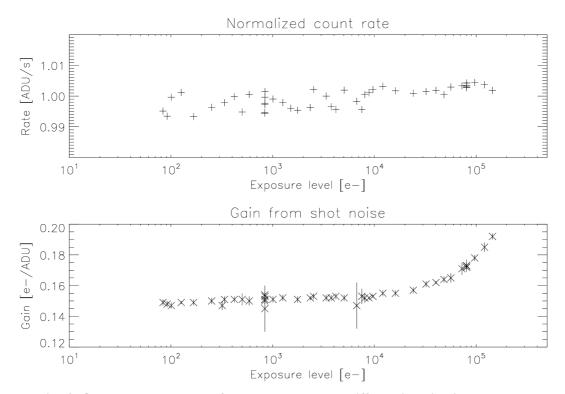
Illustration 2: Output B. Data merged from two sequences at different illumination levels.
