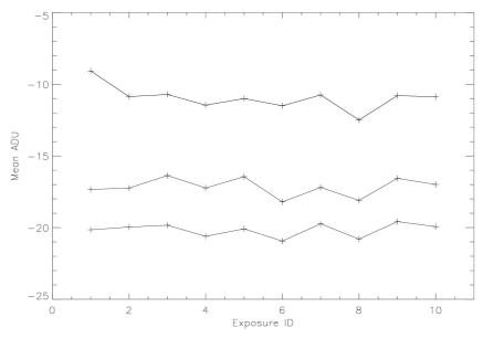
Illustration 9: Average background at the position of the three brightest saturated sources during a sequence of 10 100 sec darks.
