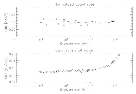
Illustration 4: Output D. Data merged from two sequences at different illumination levels.
