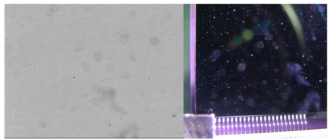
Illustration 7: Left: An approx. 900x700 section of a 550nm flatfield. Right: The corresponding area photographed with oblique illumination.
