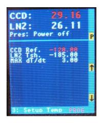
**4: Setup Reg.**: Used to alter the PID-regulator constants. These parameters are usually fitted to the current dewar before shipment.
