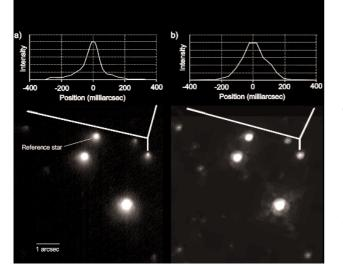
Fig. 1. The centre of the globular cluster M13 as observed with NOT/LuckyCam (left) and the Hubble Space Telescope/WFPC2 (right). A cut through the image profiles is shown at top.
