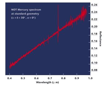
Fig. 2. NOT reflectance spectrum of Mercury for the wavelength range 400-1000 nm, calculated at standard geometry. The noise spike at 770 nm is due to the strong telluric A-band.
